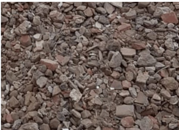
An example of our recycled 6F5 aggregate
